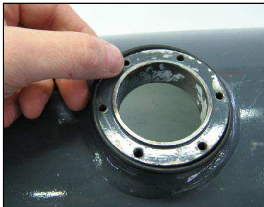
Figure 11: Placement of the O-ring gasket
