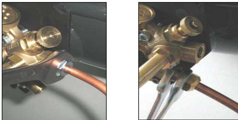
Figure 37: inlet and outlet fittings screwing 0° toroidal tank
