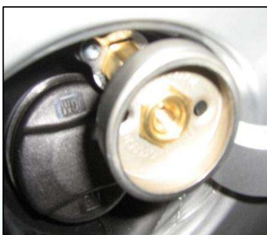
Figure 39: filling point installation
