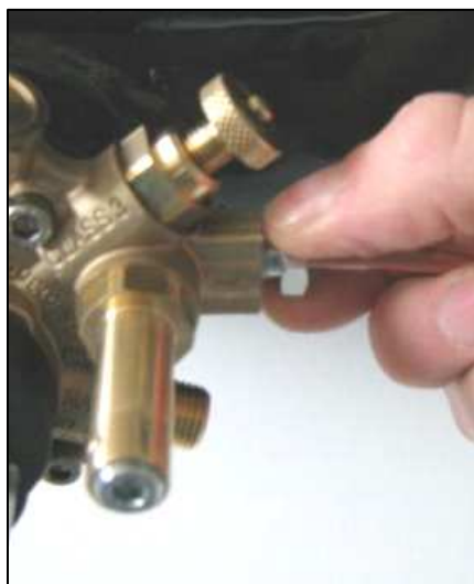
Figure 25: outlet fitting manual connection
