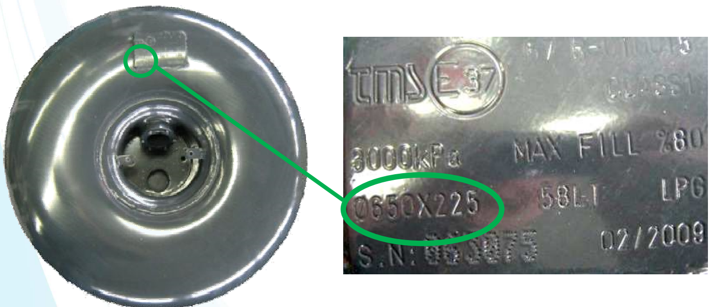
Figure 2: LPG tank size
