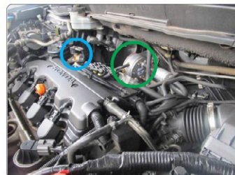
Vaporizer and LPG Solenoid, installed on a Honda CRV. Vaporizer on green, solenoid in light blue.
