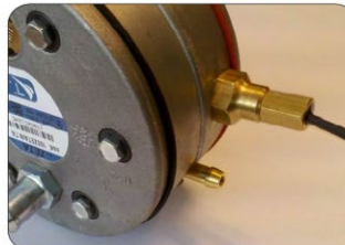
Sensor Installed. Metallic end, 15° to 25° tightened.
