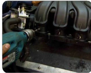
Perforating the intake manifold
