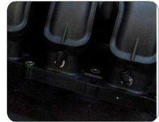
Installed nozzles (in this case, orientable)
