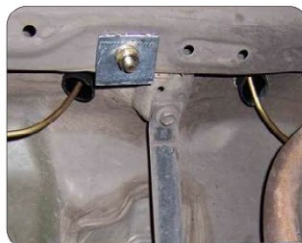
Venting pipes seen from below
