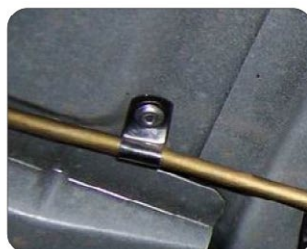
Pipe secured with the clamps provided in the kit.
