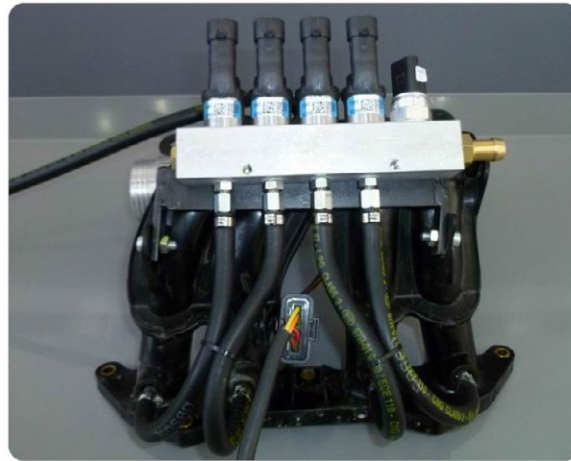
IN03 MY 09 Injector rail installed on a Peugeot/Citroën Tu3 intake manifold
