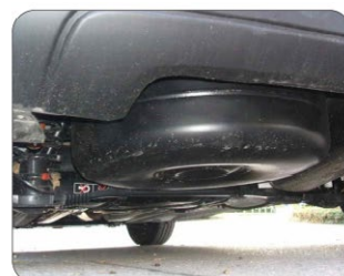
Toroidal LPG tank installed under chassis, on the spare tire compartment.
