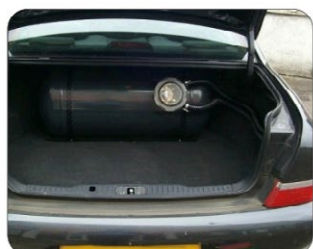
LPG tank with multi-valve, vapour box, and venting system, on trunk/bootspace
