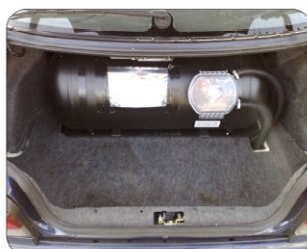
LPG tank with multi-valve, vapour box, on trunk/bootspace
