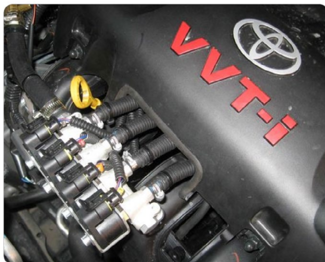
IG-1 Injector rail installed on a VVT-i engine
