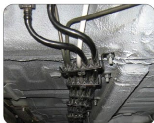
Pipes installed in a free slot of the original holders of the vehicle
