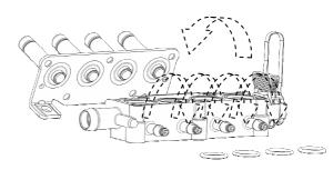
Place the 4 O-rings supplied with the repair kit.
