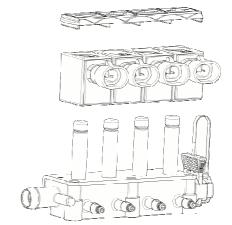
Unscrew the five screw maintening tubes in vertical position.
