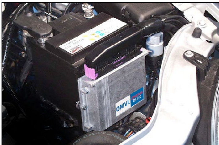
Pict. 13 Assembly of the ECU in the engine compartment
