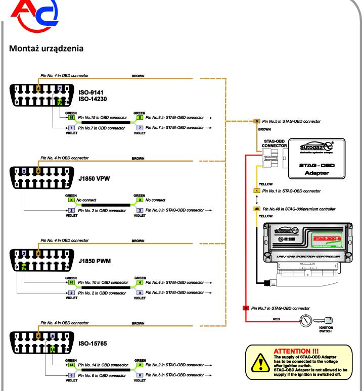
Locate the vehicle's 16-pin diagnostic connector. The connector should be located in the vehicle's cab on the driver's side or in the passenger compartment.
